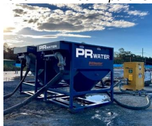
High Volume Setup SDS + 2x HB60 in parallel
