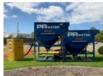
Heavy Metal Removal Set-up SDS + 2x HB60 in series
